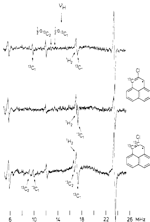
Figure 8. ENDOR spectra of 3b (toluene, 290 K) obtained when the most intense high- (top) or low-field (center) ESR component is saturated (see Figure 3, center). Bottom, ENDOR spectrum of 3bc (toluene, 290 K, center-field setting).
