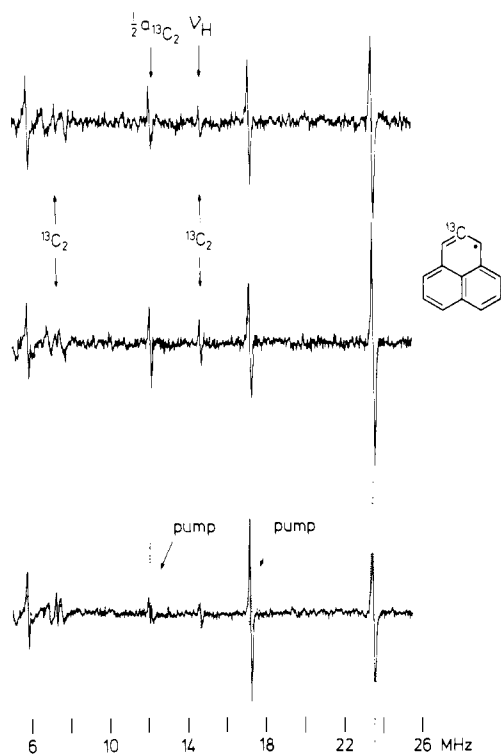
Figure 5. ENDOR spectra of 1c (toluene, 290 K) obtained when saturating ESR components assigned to this radical (cf. Figure 2, bottom): top, high-field setting; center, low-field setting; bottom, general TRIPLE spectra of 1c . The arrows indicate the setting of the pump frequency in the respective experiment.
